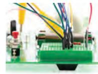
Install this small breadboard to easily conduct experiments using additional electronic components not permanently mounted on the Vernier Circuit Board 2.
