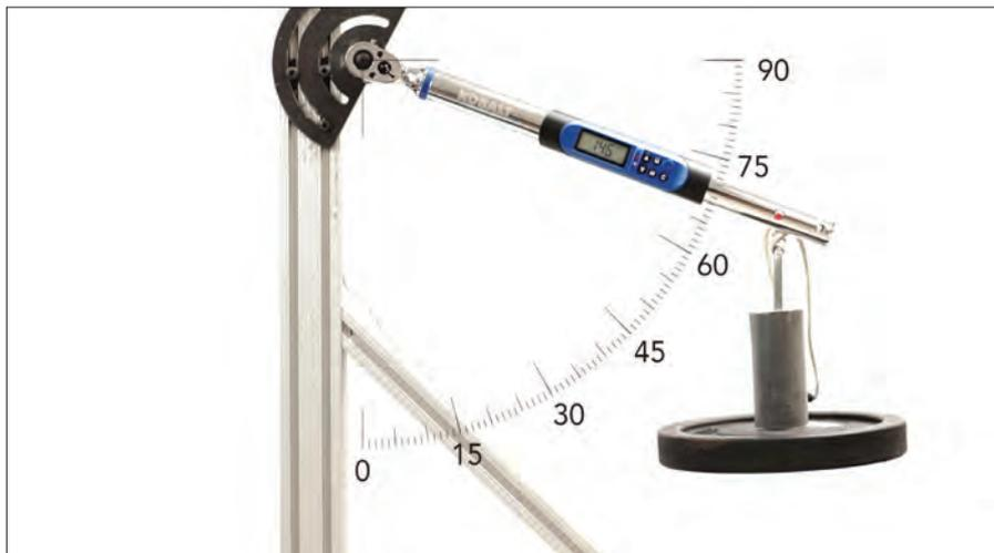
Students overlay tools onto high-quality videos to make measurements, such as in this activity where torque is calculated.
