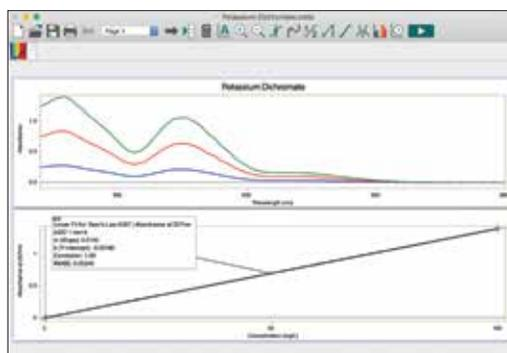
*Examining the absorbance spectrum of potassium dichromate using the Vernier UV-VIS Spectrophotometer and Logger Pro®*
